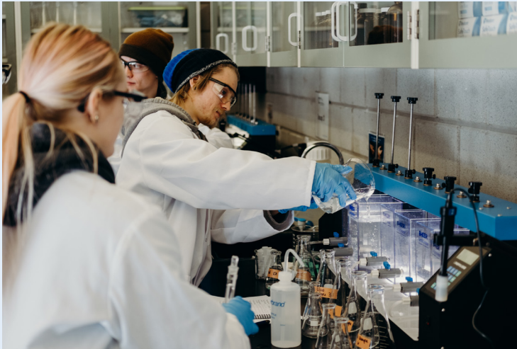
Jar testing experiments being performed for conventional treatment optimization in the WCWC laboratory
