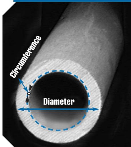
This diagram shows how to measure the diameter for a clamp.
