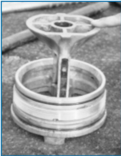
As the hydrant is closed, the upper valve plate slides up and uncovers the weep holes, allowing the hydrant to drain. As the main valve is forced away from the seat ring, the upper valve plate moves down to seal off the drain.
